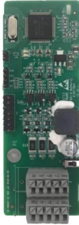
Simplified incremental PG card EC-PG507-12
