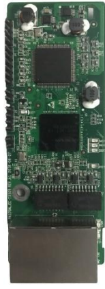
PROFINET communication card EC-TX509
