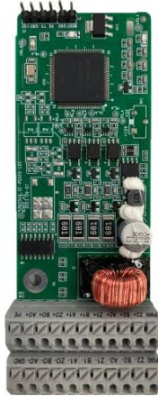
24V incremental PG card EC-PG505-24B
