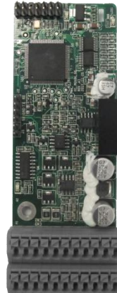
Resolver PG card EC-PG504-00
