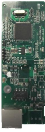
Ethernet communication card EC-TX504
