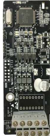
24V simplified incremental PG card EC-PG507-24
